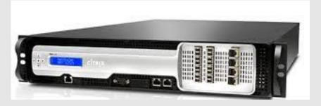
2U configuration with 4 x 40Gb/s SFP+ ports Supporting 90+Gb/s SSL/TLS encryption throughput
